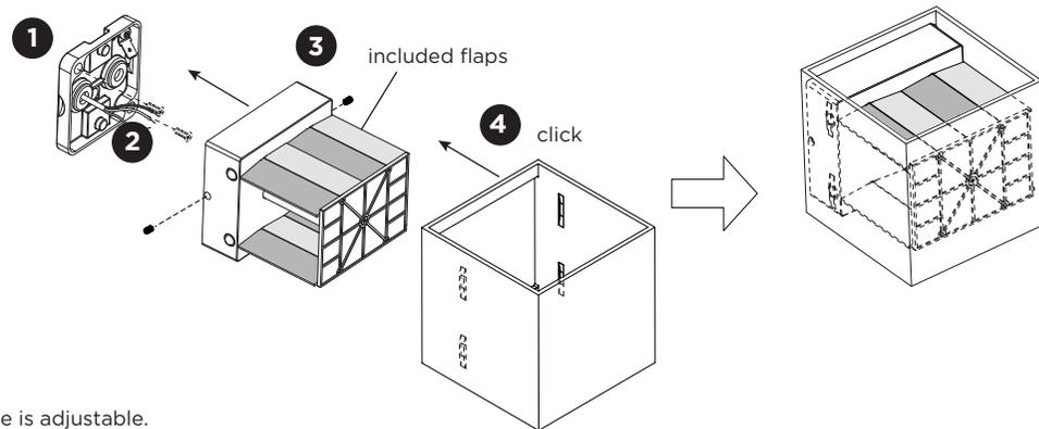
With flaps the beam angle is adjustable.
