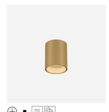
Cylindrical ceiling surface mounted downlight made from die-cast aluminium; surface Champagne; wet painted; brushed; with COB (Chip on Board) technology for maximum efficiency; phase-cut dim; light colour 2700 K; ≤ 2 SDCM (initial MacAdam); CRI ≥ 90; beam angle 30°; degree of protection IP20; Class 1; driver included; light source replaceable by Wever & Ducré or by a professional with explicit authorization; control gear replaceable by end-user;
