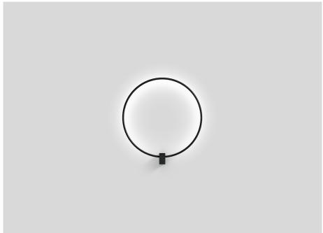
Round wall surface luminaire made from aluminium; indirect light distribution; surface Black Matt; powder coated, matt texture; RAL 9005; opal PMMA diffuser; PCB 3-step binning; phase-cut dim; light colour 2700 K; binning initial MacAdam  $\leq$  3 SDCM; CRI  $\geq$  90; 220 - 240 V; degree of protection IP20; PC1; driver included; optional spacer available for overlapping; light source replaceable by an authorized professional; control gear replaceable by end-user;
