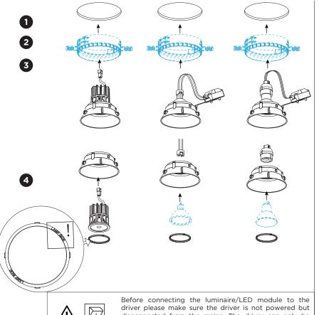
disconnected from the mains. The driver can only be powered when the luminaire/LED module is already connected. Disregarding this instruction might damage or even destroy the luminaire/LED module. powered off before
